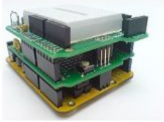
Multiple shields can be stacked. In this example the top shield contains a solderless breadboard.
