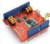
Dragino Lora Shield allows the user to send data and reach extremely long ranges at low data-rates.
